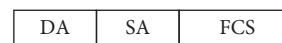
FIGURE 2: ACK frame at the data link layer is used for reliable communication.
