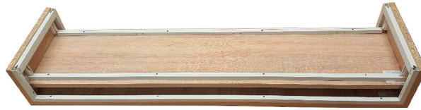
FIGURE 16: Fabricated proposed TX-coil, bottom view.
